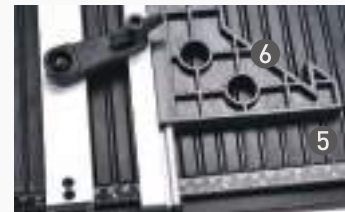
Angle Guide Plate & Micro-adjustable cutting guide
