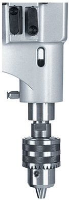
MT3 Chuck Adaptor and 5/8" Chuck (Not included)
